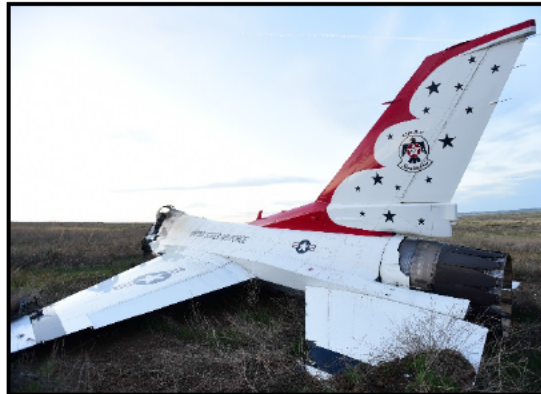
Figure 12. MA Left horizontal stab damage (Tab Z-8)
