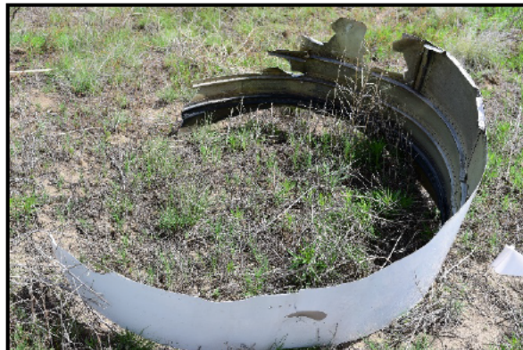
Figure 10. MA Engine bay access cover in debris field (Tab Z-6)
